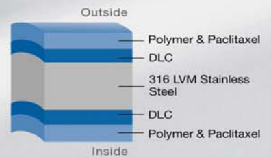
Longitudinal cut through stent strut
